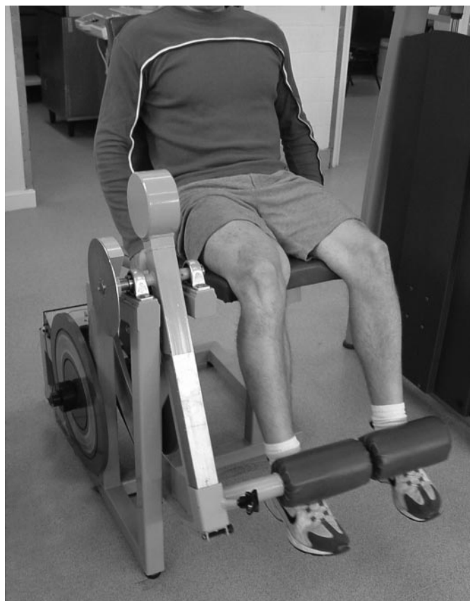
Fig. 1. Picture showing the gravity-independent ergometer used for resistance training.
