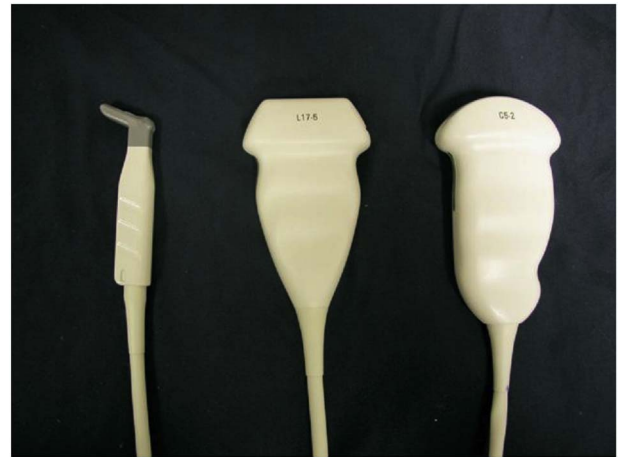
Fig. 1. Commonly used ultrasound transducers in musculoskeletal ultrasound. Left, High-frequency (15-7 MHz), small-footprint, linear array transducer, also called a “hockey stick” transducer. Center, High-frequency (17-5 MHz) linear array transducer. Right, Low-to medium-frequency (5-2 MHz) curvilinear array transducer. Both linear transducers are used for superficial imaging, whereas the curvilinear transducer's lower frequency facilitates examination of deeper regions such as the hip (Philips iU22 Ultrasound Machine; Philips Medical Systems, Bothell, WA).
